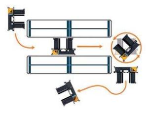
The multi-directional steering system allows the operator to choose from 12 different steering modes. It is possible to steer via the front wheels, the rear wheels or all four wheels simultaneously. This allows the truck to negotiate service aisles, travel diagonally or turn on its own axis. Must be driven to be appreciated.
