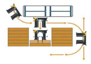
The 4 Way version offers an economical steering solution with its conventional forward / reverse travel and sideways operation. Loads are easily accessed from tight quarters. It remains highly manuevrable and the vehicle is able to turn within its own length.
